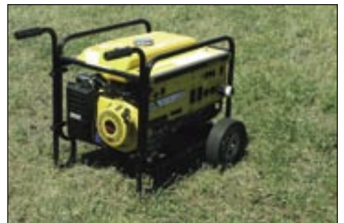
Reciprocating Engine (Generator)
